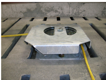
Corner wheel with protective cover
